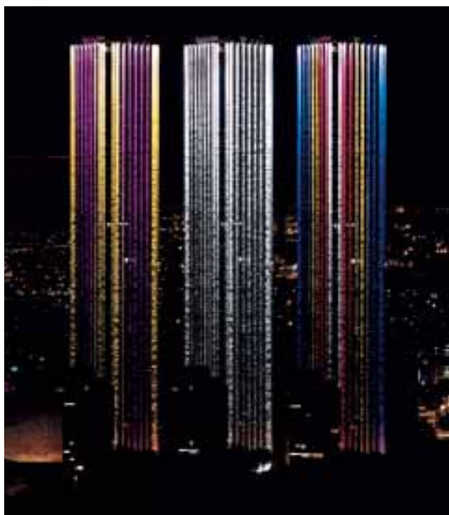
A lighting installation with XBO® 3 and 4 kW. These lamps shower the facades in eye-catching colours from spotlights mounted on the roof of the 200 meter high Bogotá Tower in Colombia.
